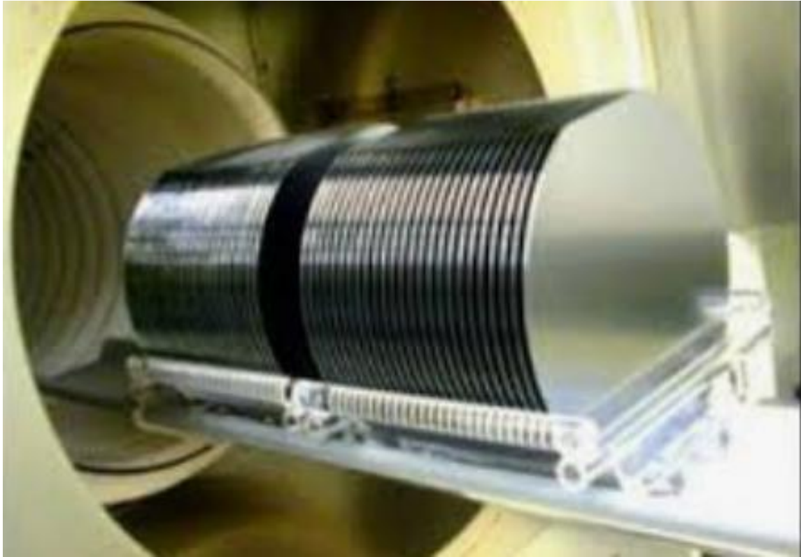
300mm wafers loading in diffusion furnace
